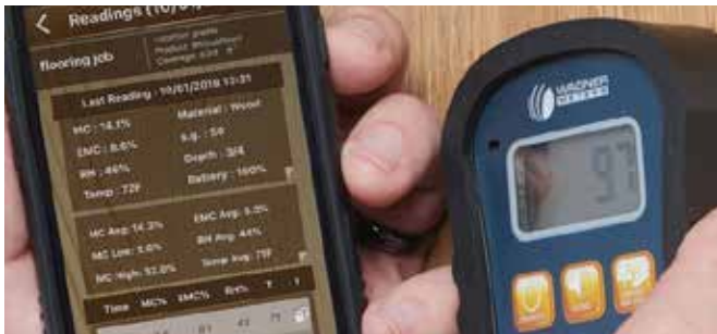
The simplest way to monitor the moisture levels in your wood is to use a handheld moisture meter calibrated for the type of wood that you are installing.
